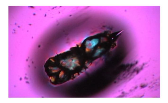
The Batch stones are a sort of defects they have to be recognised as soon as possible; in fact they are a very important witness of the "health" of melting and fining process, or in other words, of the back side of the glass furnace.
